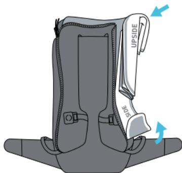
Now set the backpack upright and fold the rear part of the airbag backwards into the still open airbag compartment. You can now close the upper section zip. In so doing, ensure that you secure the burst section (shown in the centre in white) of the zip to the backpack using the corresponding hook and loop fastener. Finally, you can close the left shoulder strap and secure the zip slider using the loop provided at the end of the shoulder strap (Fig. 7.7).
